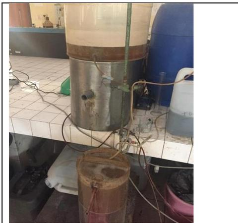
**Gambar 3** reaktor lumpur aktif (reaktor Activated Sludge /AS), V = 5 L
