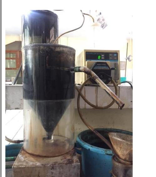
**Gambar 2.** Reaktor Upflow Anaerobic V = 5 L
